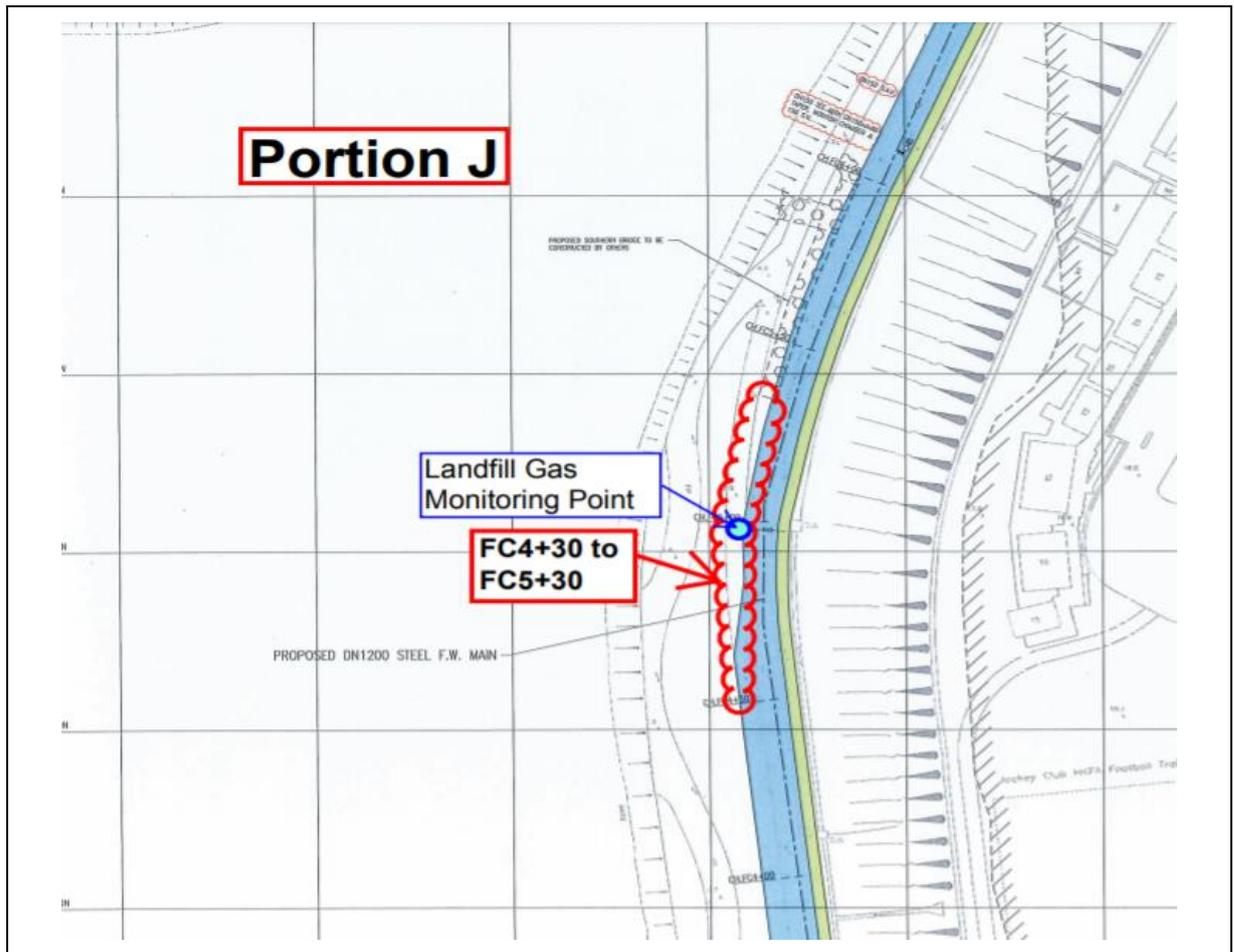
Figure 4.10c Monitoring Location – Landfill Stage 1 (FC4+30-FC5+30)
