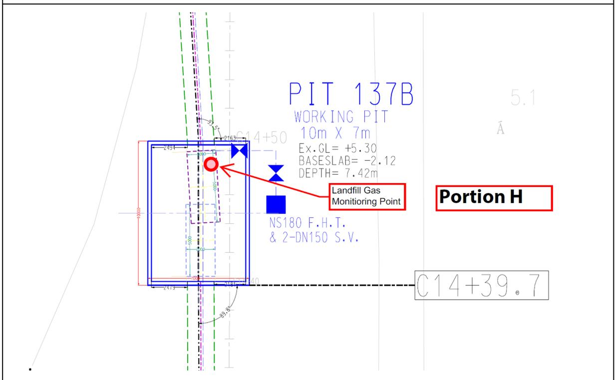
Figure 4.8b Monitoring Location – Pit 137B (137 Pit B)
